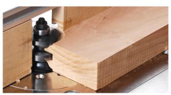
The next step is to shape the panel groove and the decorative ogee profile along the inside edges of the door frame members. Adjust the height of the bit so that the cut is centered on the stock thickness. Then position the fence tangent to the guide bearing. Now cut the ogee and groove on the frame members.
