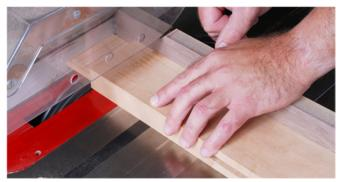
The next step is to cut the tenons on the ends of the rails. But first you'll need to cut the rails to length. To calculate the rail length, add 1" to the shoulder length for the cope at each end then add the tenon length x2.
