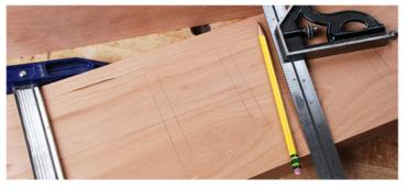
Next, clamp the stiles together and transfer the layout to the matching stile. This ensures that the measurements on the left and right stiles correspond. Now transfer the mortise locations to the edge of the stiles.
