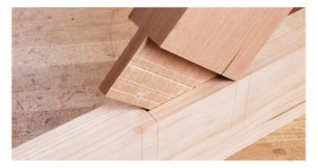
Cut the tenons for a friction fit with the mortises.
