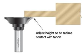
With the mortise-and-tenon joints cut you're ready to cut the cope on the ends of the rails. To cut the cope, the workpiece is guided with the miter gauge while the fence serves to limit the depth of the cope. First, adjust the height of the cope bit so that it lightly touches the tenon.
