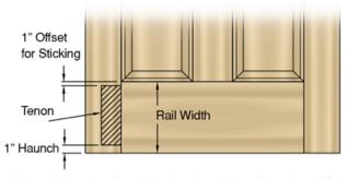
Begin by marking the stiles for the location of the rail mortises. Mark the rail width first, and then mark the haunch and the inset for the panel groove. The mortise is located between the marks for the haunch and the inset.
