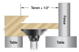
Next, position the fence. To determine the correct fence position, add 1/2" to the tenon length. The distance from the fence to the tip of the cope bit should equal that measurement.
