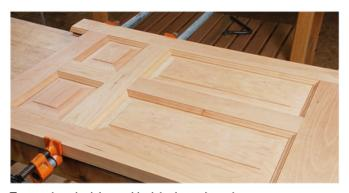
To complete the joinery chisel the haunch on the tenons to correspond with the panel groove on the stiles. Then shape the panels and fit them in the frame.
