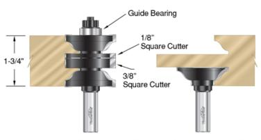
The Timberline Extended Tenon Door Bits are an effective way to produce stile-and-rail architectural doors with authentic mortise-and-tenon joinery.
